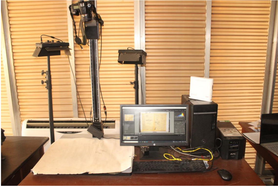
Figure 2: A camera, copy stand, two light stands and a computer system (server) with UPS used for the digitisation of Yoruba newspapers at the Kenneth Dike Library, University of Ibadan (2021).
